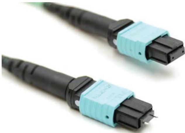
MTP Male Female MPOs are classified by the guide pins on the end of the connector, and require 1 male and 1 female to mate properly. MPO connectors use a “barrel sleeve” adapter that simply holds one male and one female MPO “plug” together. The male guide pins fit into the female holes to ensure precise fiber alignment. It is never advised to mate two female connectors two male connectors due to both insertion loss and pin damage respectively.
