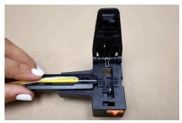
Step 3: Place fiber and cutting jig into holder until cleaver stopper.
