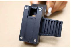
Step 2: Push the blade shelf down to the cutting position.
