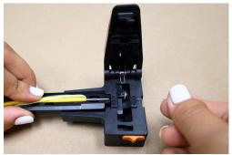
Step 5: The lid will open automatically after releasing it. Discard the cut fiber and remove the cable from the holder. Cleave is complete.
