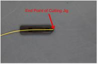
Step 5: Fix the fiber into the cutting jig. The end of remaining 900 µm tight-buffer coating should meet the end point of the cutting jig.
