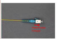
Step 8: Press the pusher forward to lock the fiber.
