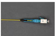
Step 9: Push the 900µm tail boot into the slot at the end of the connector.
