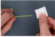
Step 4: Clean the bare fiber with the dust-free wipe.
