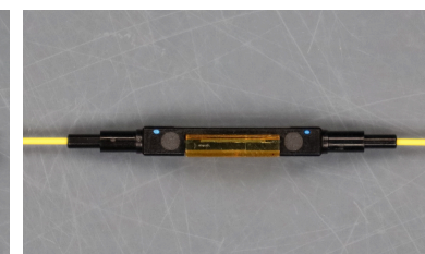
Step 9: Repeat Steps 1-8 on the other side of the mechanical splice. Press the locker (yellow) down to lock both fibers in place, completing the assembly.
