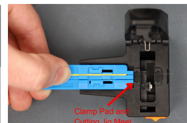
Step 5: Slide the cutting jig in the holder slot of the cleaver until it meets the clamp pad. Cleave fiber.
