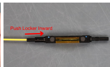
Step 8: Push the locker (black) inward to lock the fiber.
