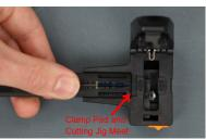
Step 6: Slide the cutting jig in the holder slot of the cleaver until it meets the clamp pad. Cleave fiber.
