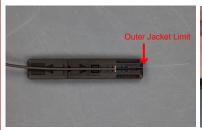
Step 5: Extend the cutting jig out entirely. Fix the cable into the cutting jig. The outer jacket must meet the outer jacket limit.
