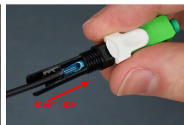
Step 9: Insert the fiber into the connector until the fibers meet inside—you'll feel resistance. Push the drop cable jacket into the slot with teeth at the base of the connector.
