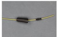
Step 1: Put the tail boot and the 900µm tail boot onto the cable.
