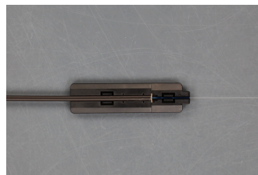
Step 7: Fix the cable into the cutting jig. The outer jacket must meet the outer jacket limit. The 250µm acrylate coating should meet the end of the cutting jig.
